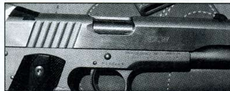
An effective dehorning job and a lowered and flared ejection port are just two of the niceties one finds on the Para CCW.
