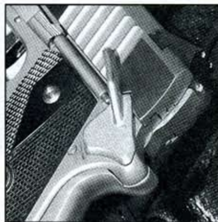
When applied the thumb safety locks the slide and disengages the trigger.
