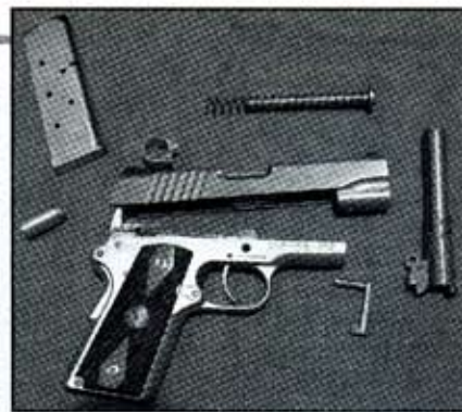
Field stripping the CCW is done the same as any other 1911.
