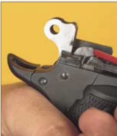
A simple steel riser acts against a frame-mounted plunger to block the firing pin.
