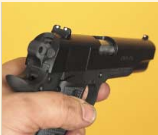
Sights on the new Para-Ord P14 LDA are the basic three-dot, square-notch and blade style.
