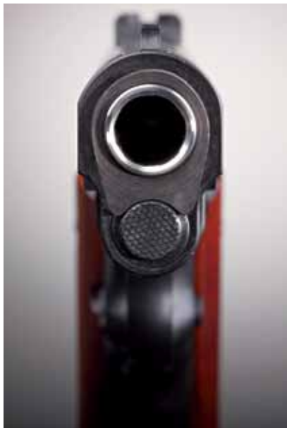
In keeping with the traditional themes, a stock bushing and spring tube were used on the 1911.
