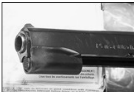
Repeated rapid fire only temporarily discolored the slide.
