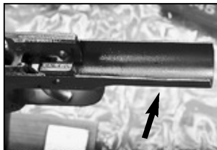
At about 1500 rounds, this side of the dustcover warped.
