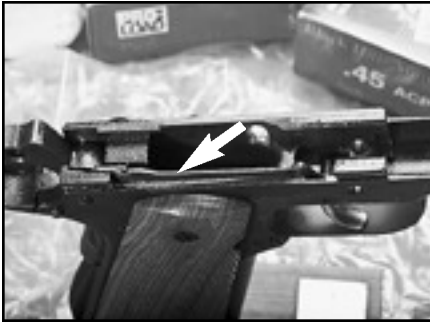
The LDA uses a drawbar to activate the firing mechanism.
