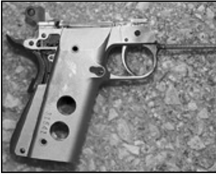
Factory cutaway LDA shows the inner workings of the action.
